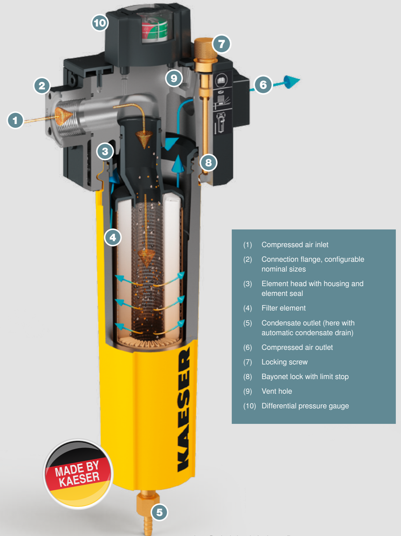
Image: Functional schematic of coalescence filter
